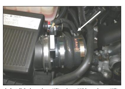
**4.** Install the hump hose (#3) and two #60 hose clamps (#5) on the Mass Air Flow sensor as shown. Leave the clamps loose for now.
