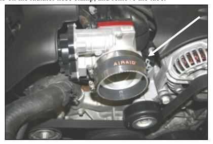
**5.** Install the coupler (#4) and two #64 hose clamps (#6) on the throttle body as shown. Leave the hose clamps loose for now.
