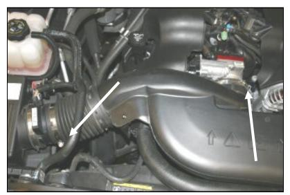
2. Loosen the hose clamps on both ends of the factory intake tube.
